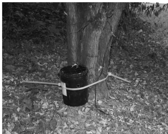
Figure 1. Ovitrap used in the Emilia-Romagna monitoring network since 2010 (CAA14).
