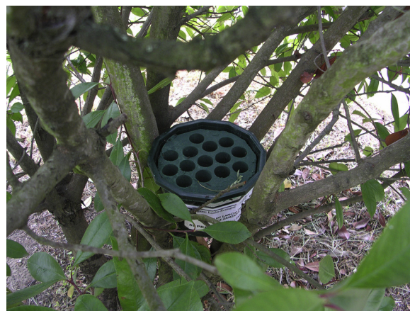
Fig. 1. Device to release sterile male pupae. The device consists of a conical green dark plastic container with a base diameter of 13.5 cm, top diameter of 17.5 cm and height of 12.5 cm in which a polyurethane sponge drilled with 2 cm diameter holes was fitted. The sponge was soaked in the desired sugar solution just before field deployment. The newly emerged males must go through the holes to take flight.
